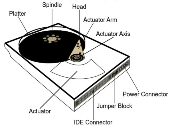
You also needed to point out that the lateral movement of the arm to reposition the heads (seeking) is the major source of latency.
